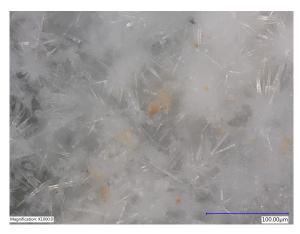
Figure 3: Crystal growth in cracked concrete (Magnification x I 000)
